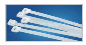
One-piece design molded of fungus-inert, self-extinguishing, white opaque virgin nylon. Can be used in temperatures ranging from -40 F to 185 F. Bent tip allows the user to insert the tip easily and quickly into the self-locking head. Meets all applicable military specs. U.L. approved, Nylon 6/6
